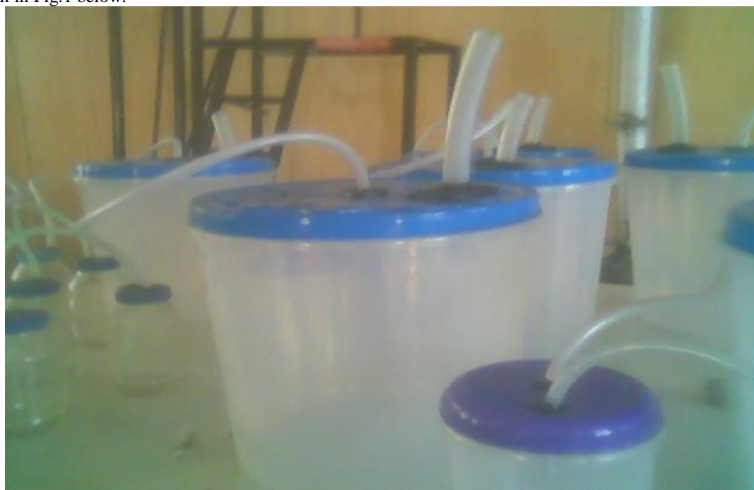
Fig. 1: A newly Constructed Plastic Bio-digester
